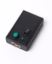
The Phoenix™ 2.5 Program Controller (NSN: 5855-01 -452-0079) is designed to support the command coding of one or more Phoenix 2.5 Beacons (NSN: 5855-01-452 -9877) with speed and precision.
