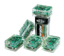
**Velux™ 2** is a Short Wave Infrared (SWIR) signaling beacon developed specifically to emit a flash pattern signal that can be synchronized with other Velux 2 beacons so they flash in unison.
